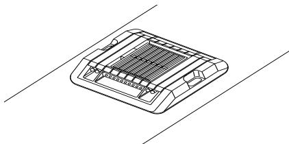
GB Fixing by embedded anchor
