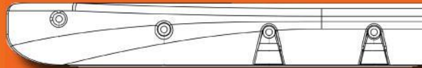
Kerb Orca RH End Section 150mm breed x 1000mm lang Gewicht 9,0 kg 4 bevestigingen
