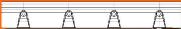
Kerb Orca Middle Section 150mm breed x 1000mm lang 100mm hoog Gewicht 11,0 kg 4 bevestigingen
